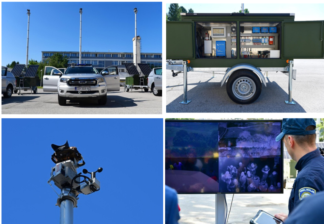
Figure 29. Mobile surveillance systems (camera system FLIR). Showcased in press releases on July 6, 2021, and August 30, 2024. Accessible here and here .
